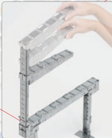
Cantilever brackets are fully adjustable and require no tools to install. Slide bracket up or down the vertical support and lock tabs into position.
